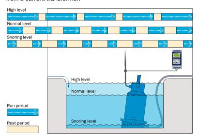
Different water levels for starting the pump can be entered via the control panel. The Emotron DCM then uses an algorithm to calculate the appropriate run and rest periods. Pump operation is automatically adapted to the pit filling rate, minimizing energy consumption and component wear.
